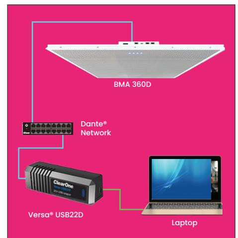
Connect the BMA 360D and Versa USB22D to a network using standard Cat 6 cables.
