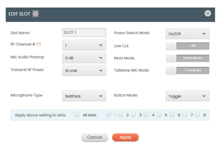
Edit each slot by clicking on the edit button for each slot. You can choose the frequency by clicking on the RF channel dropdown box. You can edit other parameters here, also.
