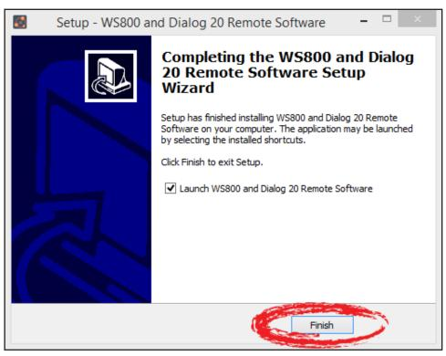
The software launches and starts to initialize. Upon startup, the software attempts to install and checks the status of the Receiver USB, Transmitter USB CDC (Communication Device 7 DOC-0581-001 User Manual Dialog 20 USB Microphone System Remote Software Class), Transmitter USB Boot loader, and DIALOG 20 USB drivers. This requires administrative privileges.
