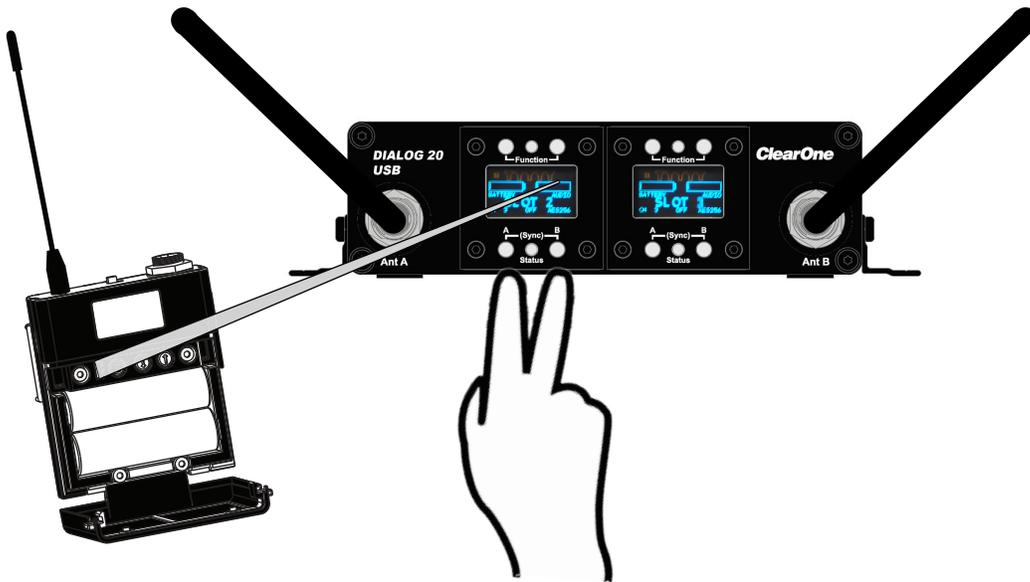
**Note:** The transmitter and receiver are assigned a new, random AES 128-bit encryption key every time they are synced.
