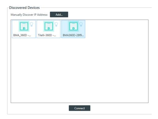
If multiple BMA 360Ds are present on the network, you can identify each by clicking on the Locate lightbulb icon. This will cause the corresponding physical BMA 360D's LED bar to flash green until the Locate icon is clicked again, or the Locate Timeout period has expired.
