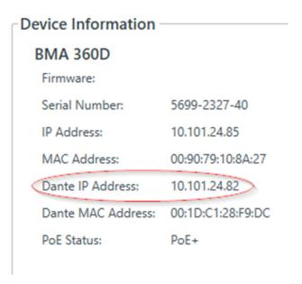
Audio routing to and from the BMA 360D is done via Dante Controller. Be sure that you have the BMA 360D and at least one other Dante enabled device, such as a DSP or Dante Virtual Soundcard attached to your Dante network prior to beginning configuration and routing. Use the Dante Controller software on your computer to verify that your BMA 360D appears on the Dante network's device list with the Device Name assigned in the Device Settings panel.
