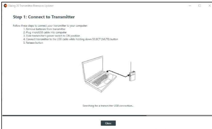
2. Using a USB cable with a Mini USB connector on one end (to connect to the D20 transmitter) and a Type A USB connector on the other end (to connect to a PC), connect the DIALOG 20 Transmitter to the PC where CONSOLE AI is installed.
