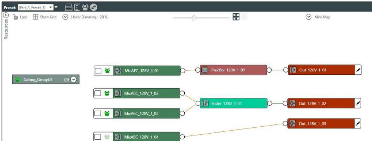
2. To add a standard reference to an output channel, click the pencil icon on the right side of the output channel icon:
