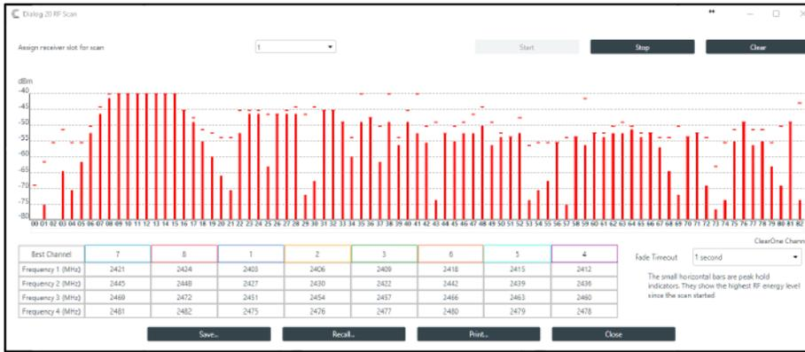
6. Results are shown at the bottom of the screen, with the best channels (those with the strongest signal) ordered from left to right, showing you the best possible channel in your environment:
