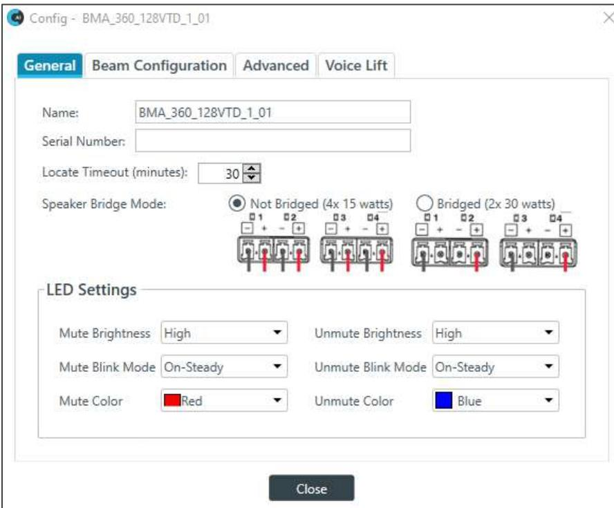
**Note:** The system displays the dialog box shown above, which includes a tab for **Voice Lift**, **only if you have already allocated** a BMA 360 Voice Lift resource.
