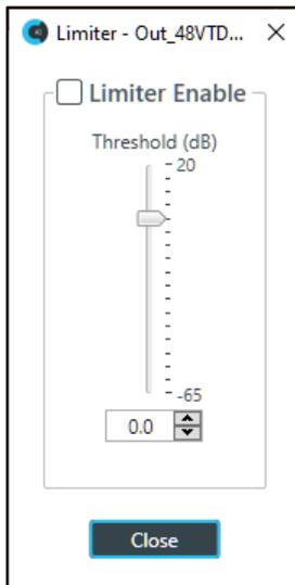
28. To activate the limiter, click the **Limiter Enable** check box.
