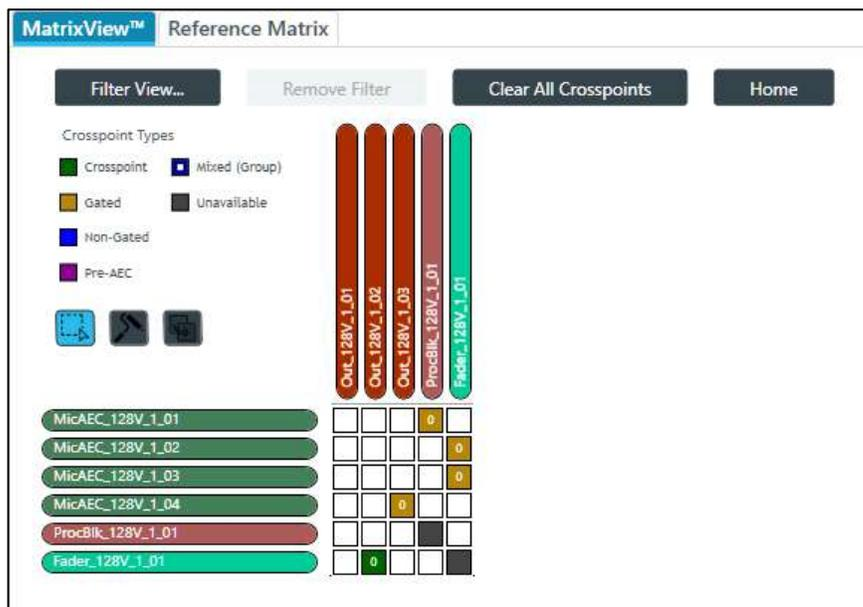
channels, have both inputs and outputs, so they appear as both a row, for the input, and as a column, for the output.
