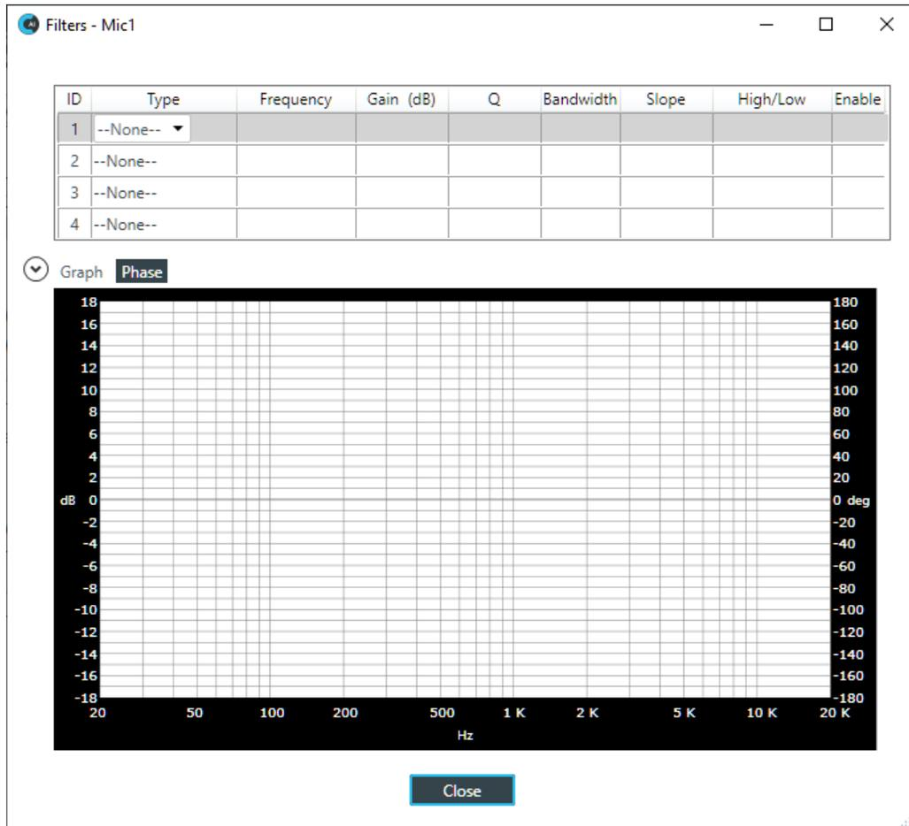
20. For one of the available filters, choose a filter type from the Type drop-down list (see the table below for a brief description of the available filter types).
