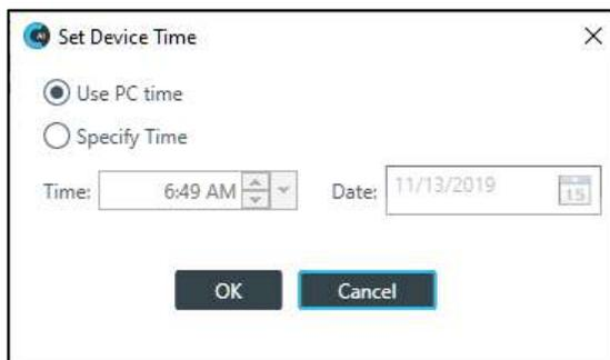
4. To use the system time from the computer running the CONSOLE application, select **Use PC Time**.
