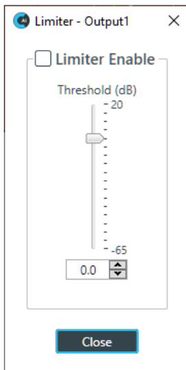
11. To activate the limiter, click the **Limiter Enable** check box.
