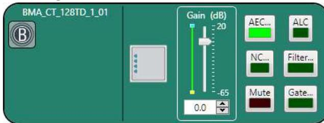
4. Click the BMA CT Config button (the button at the left side of the channel properties block that looks like a BMA CT) to change the Config settings.
