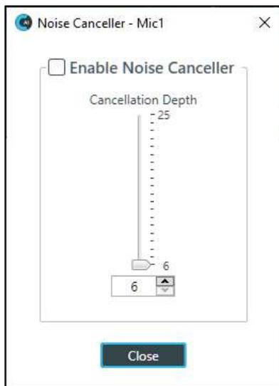
15. Check the **Enable Noise Canceller** check box to turn on NC.
