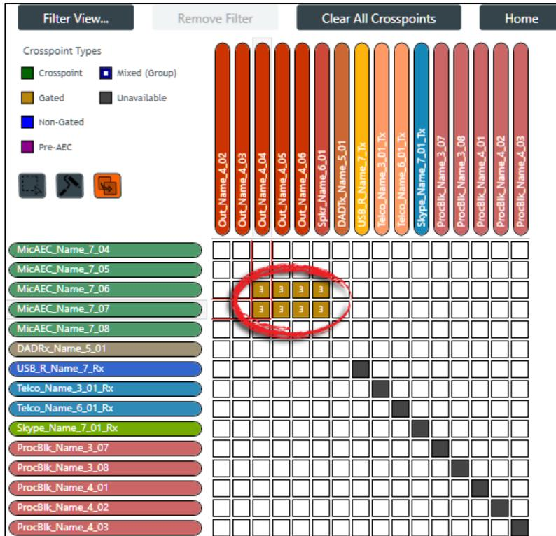
In this example, the first crosspoint touched, was the one circled in the Before image. Then the pointer was dragged across all the crosspoints circled in the After image. Notice that the crosspoint type and the attenuation value of 3 of the crosspoint circled in the Before image have been copied to all the touched crosspoints.
