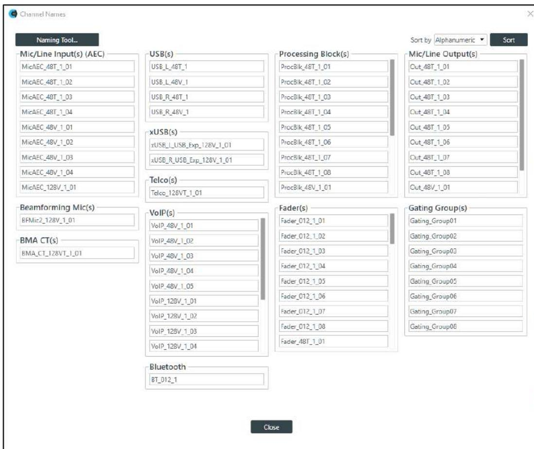
2. (Optional) To change how channels are sorted (alphanumerically or by device and connection), choose an option from the Sort by drop-down list at the top of the Naming screen and then click Sort.
