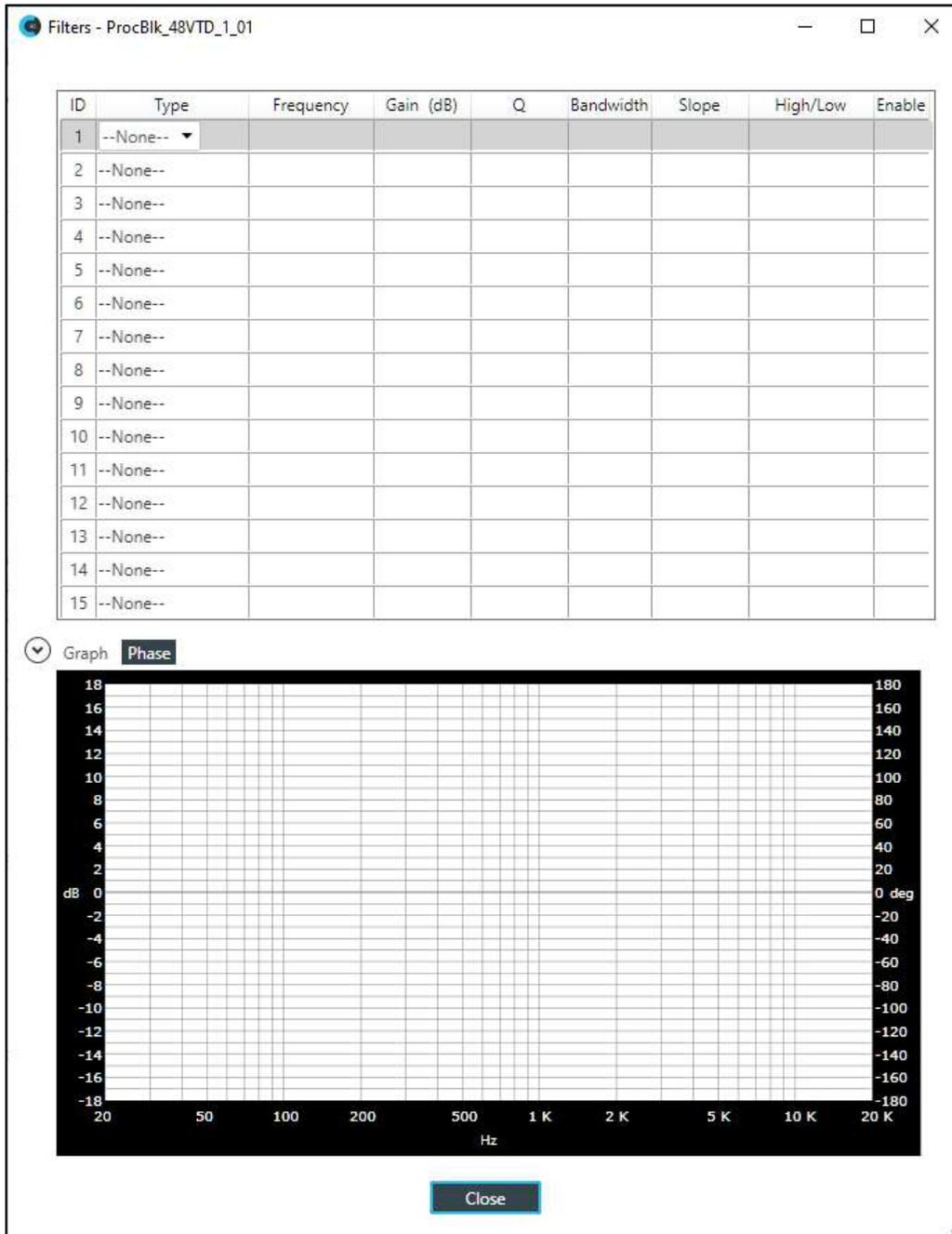
7. For one of the available filters, choose a filter type from the **Type** drop-down list (see the table below for a brief description of the available filter types).
