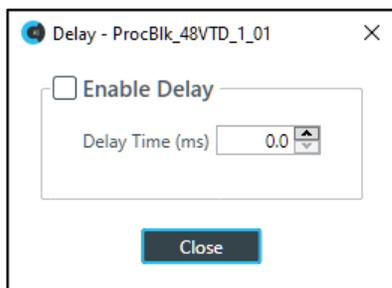
13.Check the **Enable Delay** check box to turn on the delay.
