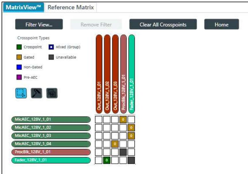
Inputs appear as matrix rows and outputs appear as matrix columns. Some channels, such as a processing block channels, have both inputs and outputs, so they appear as both a row, for the input, and as a column, for the output.
