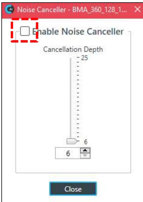
Check the **Enable Noise Canceller** check box to turn on NC.
