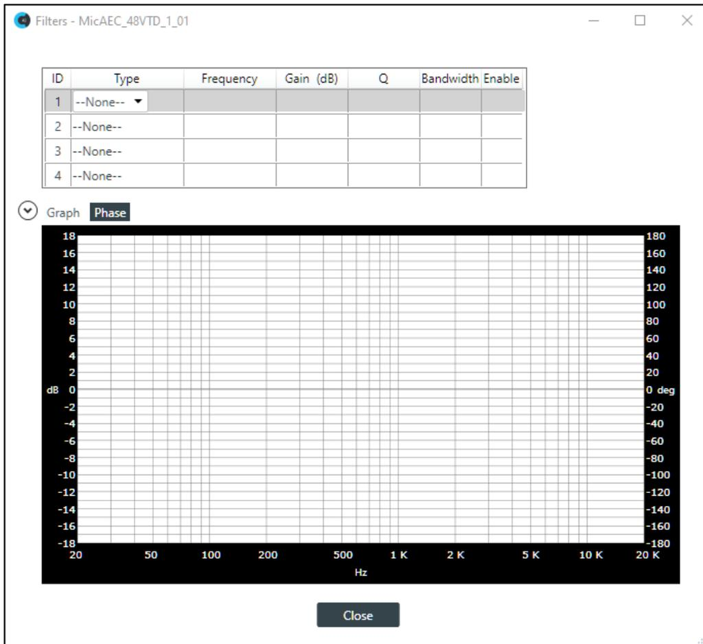
22. For one of the available filters, choose a filter type from the Type drop-down list (see the table below for a brief description of the available filter types).
