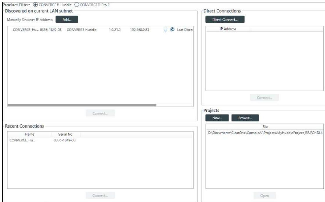
All discovered Huddle devices are listed under **Discovered on current LAN subnet**. Devices that have been connected to the CONSOLE recently are shown under **Recent Connections**.
