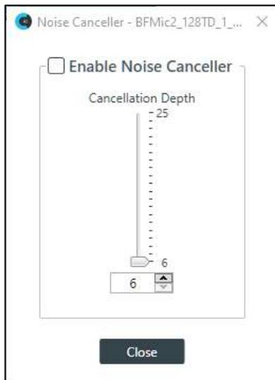
13. Check the **Enable Noise Canceller** check box to turn on NC.
