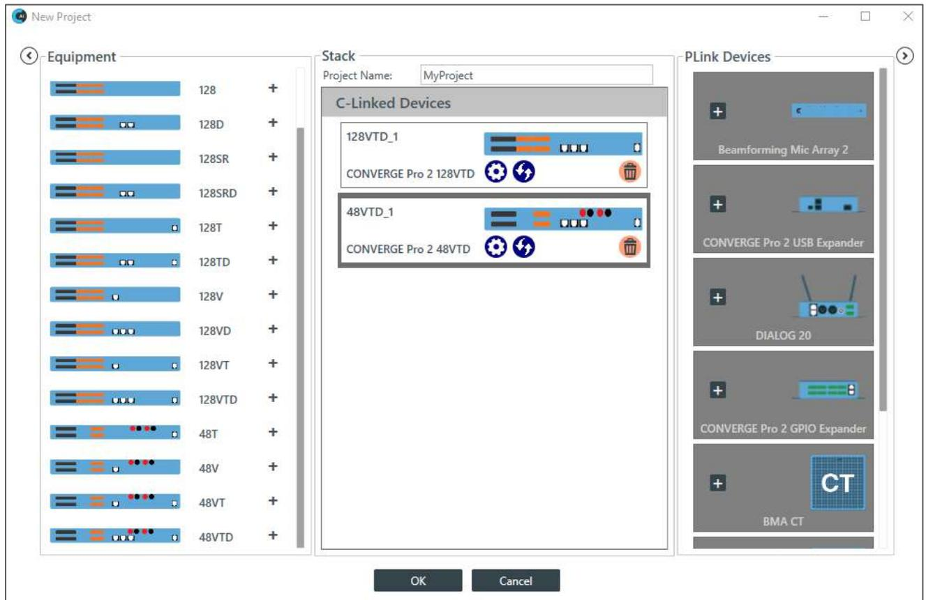
On the right of the screen, under P-Link Devices, add the BMA2 by either of two methods:
