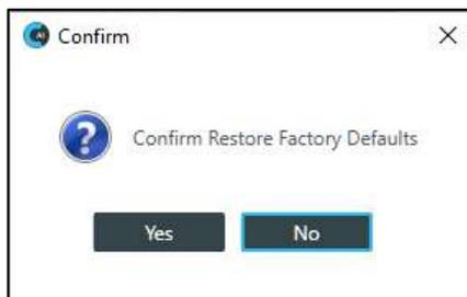
**!** **Important:** Restoring the factory defaults for a device removes all settings you have configured for the device.
