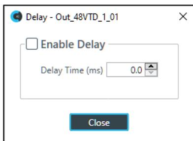
18. Check the **Enable Delay** check box to turn on the delay.
