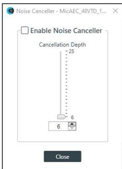
17. Check the **Enable Noise Canceller** check box to turn on NC.
