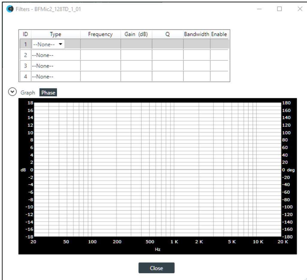
19. For one of the available filters, choose a filter type from the Type drop-down list (see the table below for a brief description of the available filter types).
