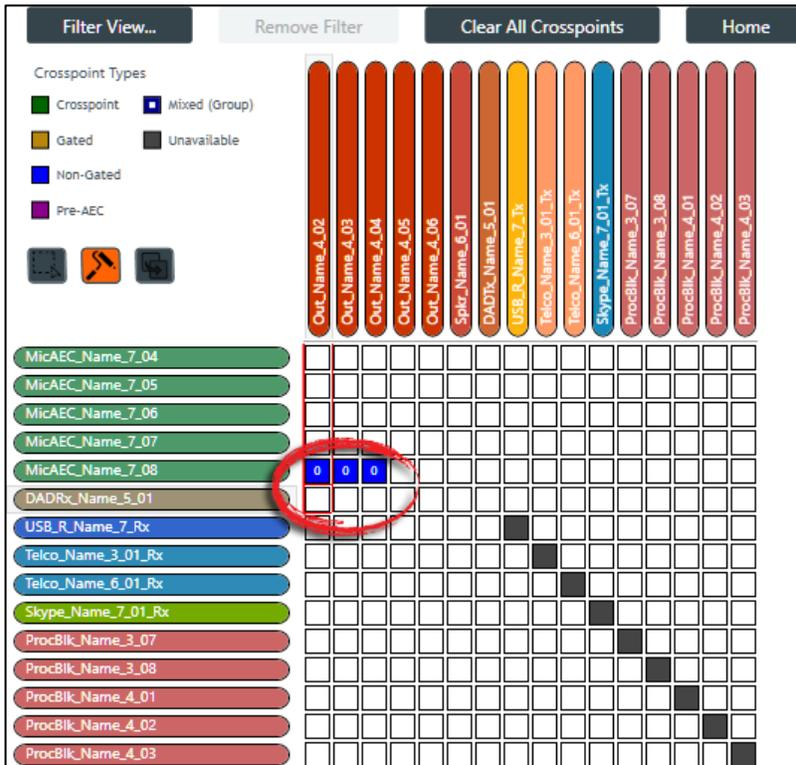
Notice that the crosspoints in the MicAEC\_Name\_7\_08 channel row have been changed from “Gated” to “Non-Gated” while the crosspoints in the DADRx\_Name\_5\_01 channel row have been changed from “Crosspoint” to blank (no crosspoint). That’s because each crosspoint touched was changed to the next available type.
