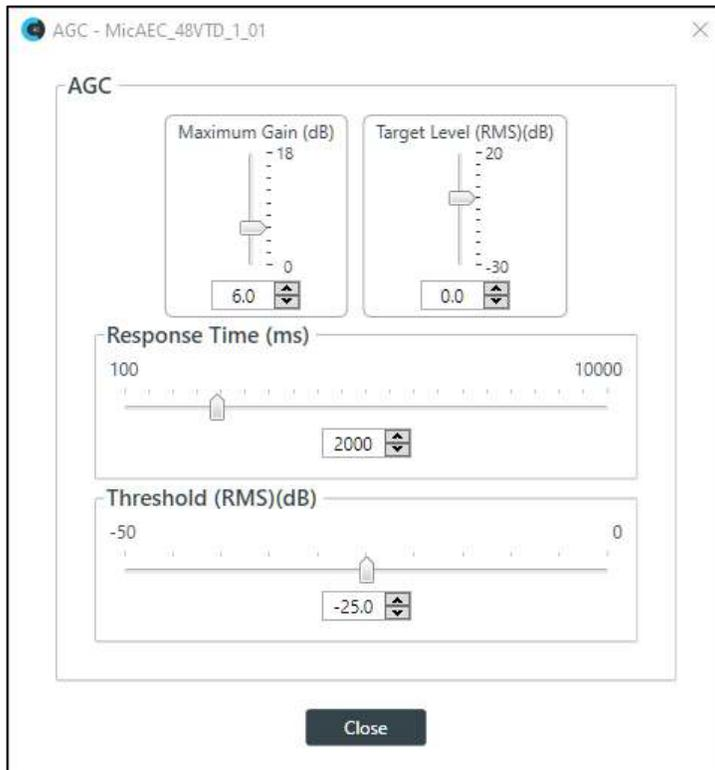
28. Use any of the following methods to change the Maximum Gain, Target Level, Response Time, or Threshold (options described in the table below):
