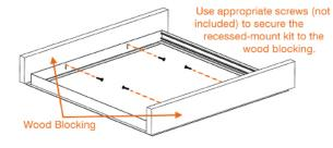
Warning! Wood blocking must be independently supported by building structure.
