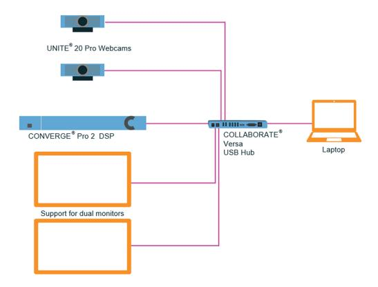
With ClearOne's easy and driverless USB interface, simply connecting your laptop to the Versa Hub enables you to pass audio to and receive audio from your CONVERGE Pro 2 audio DSP. Just select the detected ClearOne USB device in Windows or from within the audio settings of your favorite conferencing software.
