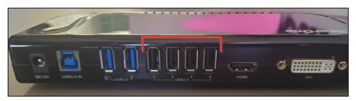
Using a USB 2.0 Type A to Type B cable, connect this port on the CONVERGE Pro 2 DSP to one of the USB 2.0 ports on the COLLABORATE Versa Hub.
