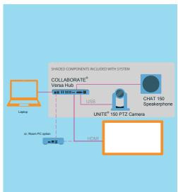
Flexibility for BYOD room systems USB 3.0 or USB 2.0 compatibility, with 4 USB 2.0 ports (with one port for smartphone charging function) and 2 USB 3.0 ports.
