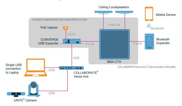
Versa Lite CT using room PC and displays, with optional ClearOne peripherals— COLLABORATE Versa Hub, choice of UNITE conferencing cameras, and Wall-Mount Bluetooth Expander
