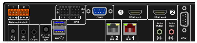
The VIEW Pro E110 Encoder has exactly the same input and output connectors on the back of the unit as the E120, but with only one 1 HDMI input connector instead.
