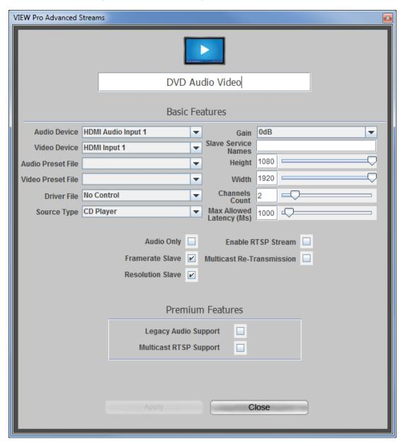
**Audio Device** – The physical input port for the audio stream.
