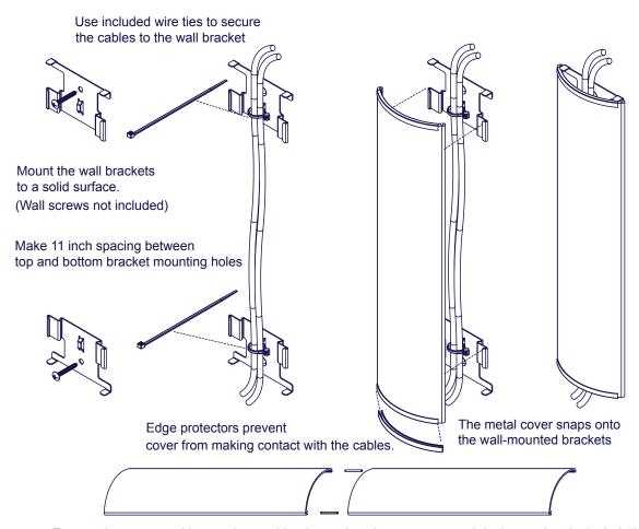
Two sections or more kits may be combined to make a longer raceway. Join them using the included spring pins.
