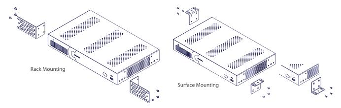
The VIEW Pro encoder can also be surface mounted using the optional Wall Mount Kit (910-0002-002) with surface-mount ears that attach to the encoder to facilitate mounting.
