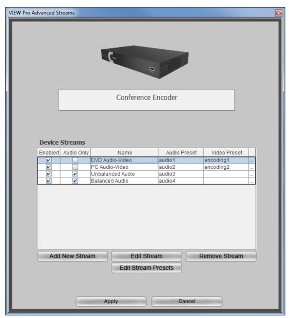
This screen allows the addition, editing and deletion of device streams for the encoder. When a new stream is added, it can be selected to then edit the stream and edit the stream presets.
