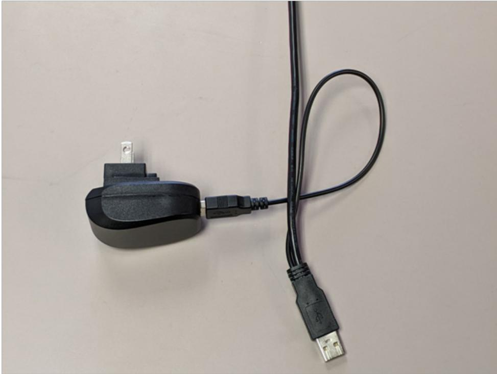
Option 2: Attach one end of the USB A to USB micro A cable supplied with the ClearOne 10 meter and 30 meter USB extender cables to the slot on the side of the main USB A connector, and connect the other end of that cable to a standard USB wall wart power supply.
