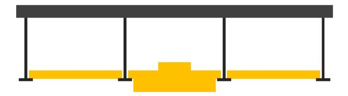
See also Claim Const. Hrg. Tr. at 72:19-73:4. In the image above, the middle tile is integrated with a BFMA, which could be located partially below the plane of the ceiling and partially above it—that is, partially in the drop space.
