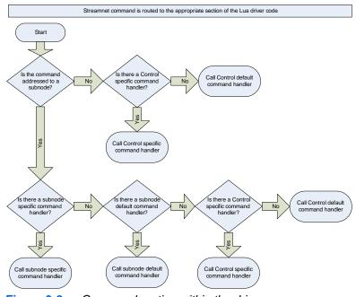
Figure 3-2 Command routing within the driver
