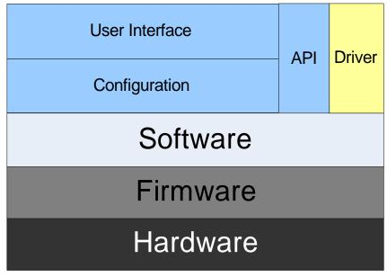
Figure 1-1 DigiLinX Hardware/Software model
