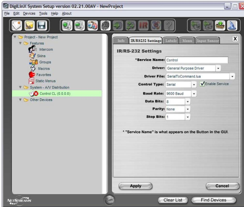
Send configurations to all devices, and DigiLinX will be ready to receive commands through the ControLinX.
