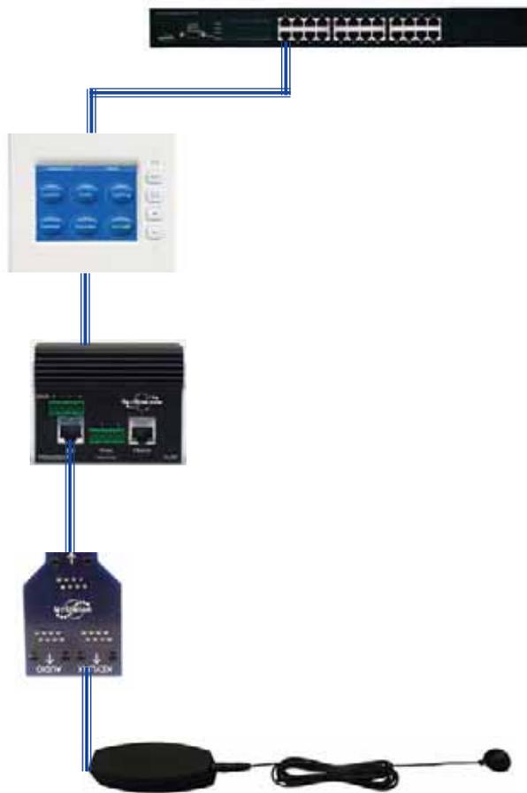
**Figure 4-6** SpeakerLinX, IRLinX, and TouchLinX configuration
