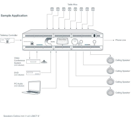
Speakers Ceiling mnt (1 pr) LS6CT 6' W/Transformer Packaged 910-151-001 Cable Spkr 18 AWG Clear C-240 50' 693-153-050 Cable Assy XLR 3-pin F To Euro 3-pin F 24" 830-151-800 Mic Kit Uni Table Top W/Cable 910-103-161
