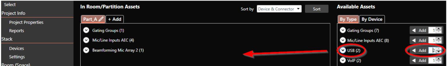
11. Add a VOIP channel. As noted earlier, the VoIP interface must be configured under Device Settings.
