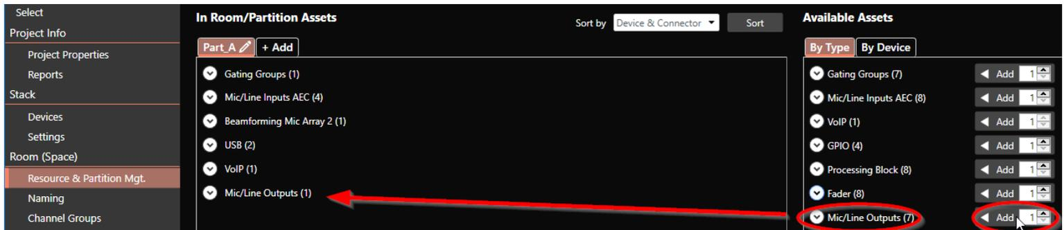
13. Add an AEC reference. Open up this output and click Add Standard to add a standard AEC reference to this output.
