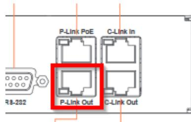
3. Connect the other end of this cable to the P-Link In port on the BFM2.
