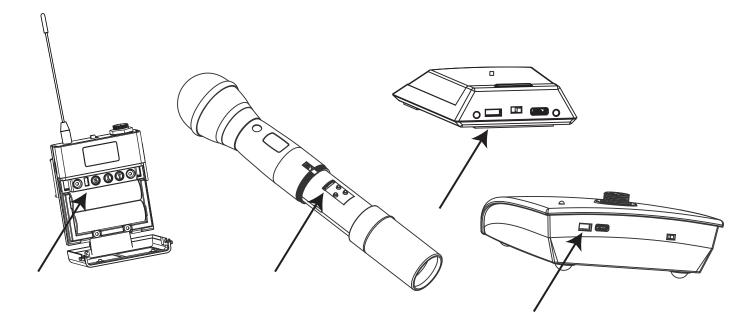
2. Hold the transmitter about 6 inches from the corresponding receiver module with the IR sensor aimed at the receiver module. **NOTE: You cannot resync if more than one transmitter is broadcasting on the resync channel.**
