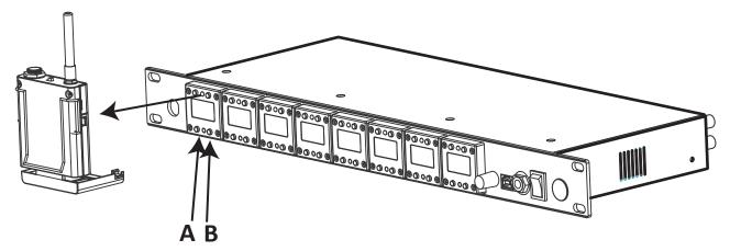
3. Simultaneously press the two buttons (A & B) on the bottom of the corresponding receiver module to start sending the IR signal. "SYNC'ING" shows on the receiver OLED when the IR signal starts. "SYNC OK" shows when the sync is successful. Repeat the procedure if the receiver display shows "SYNC FAILED". It is not necessary to press any buttons on the transmitter during the procedure.
