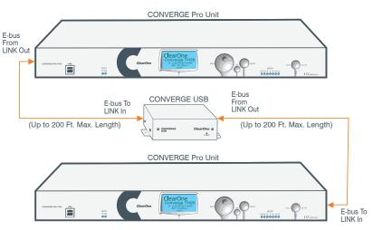
**Note:** Link Channel Selection, Routing and Audio Control are NOT required when the CONVERGE USB is used only as an E-bus extender with no USB connection.
