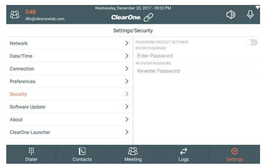
3. To turn on security for the Settings, tap the Password Protect Settings switch.
