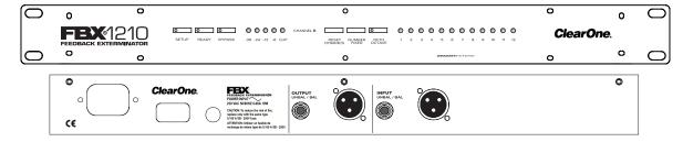
back. This unique one-Hertz resolution enables the FBX to control feedback with transparent filters that are ten times narrower than graphic equalizer filters, which can only muster 31 bands to place their very wide filters. Feedback frequencies are single tones, and that means there can be almost 20,000 places for them to occur in the audio spectrum. The Sabine FBX places filters effectively and accurately.
