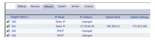
4. Select a different NIC than the one you are currently connected to. Click its name to open the configuration page.
