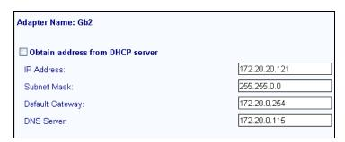
5. Assign a static IP address by entering IP Address, Subnet Mask and Default Gateway. DNS Server is optional, however, if configured it will allow you to switch between ClearOne web applications with no need to login each time.
