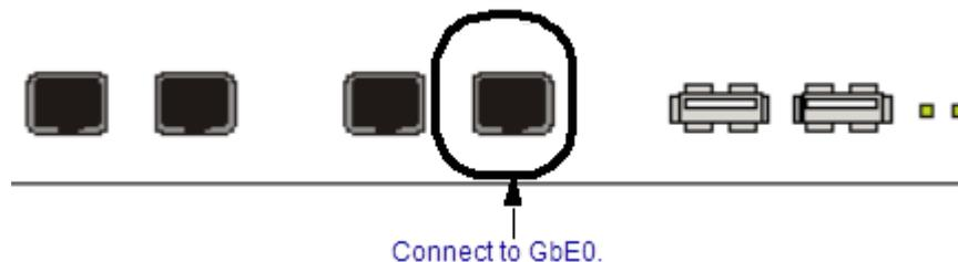
2. To access the Collaborate VCB unit from another computer initially, the two systems must, belong to the same network segment, at least temporarily. That means that the first three fields of the address and the subnet mask must be identical.
