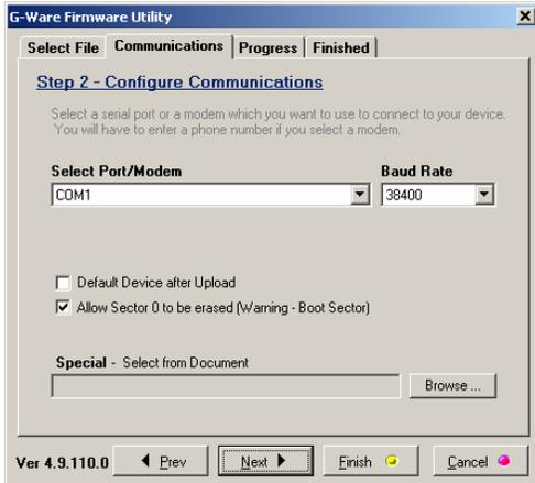
**Note:** The boot code update could take up to a minute per unit. The firmware upgrade will take approximately 5-15 minutes per unit depending on baud rate. During this time it is important not to interrupt the upgrade process or remove the cable.
