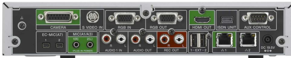
Plug the black connector labeled “Mono In” into the **AUDIO IN (L)** jack. Then plug the red and white connectors labeled “Video Codec” into the **AUDIO OUT (R)** and **(L)** jacks.
