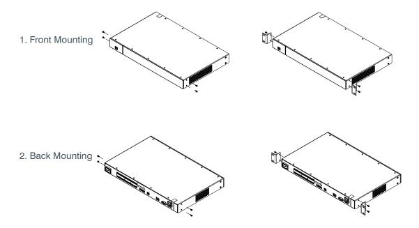
Mount the unit by securing the rack-mount ears to two posts or mounting strips in the rack using the four screws and washers provided. Because the rack-mount ears support the weight of the entire chassis, use all four screws and washers to fasten the two rack-mount brackets to the rack posts.
