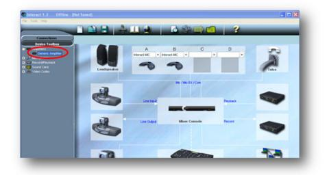
Open the Device Toolbox, open Amplifiers, and select the Generic Amplifier. With your mouse, grab the Generic amplifier icon, drag it and drop onto the correct output.
